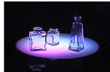
Figure 2.6 MusicBottles create an interactive surface with RFID tagging technology
