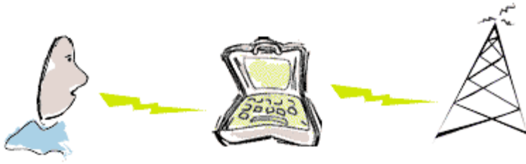
Figure 5.17 In the third architecture, devices talk to local base stations (like computers or repeaters) within rooms. Signals have to travel about 20 meters.
